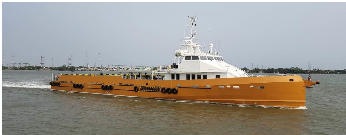
FPSV 55w: Fast Pax Supply Vessel de 55 m / hydrojets
